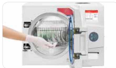
EZ9Plus loaded with 2 stainless steel trays and optional pouch rack
